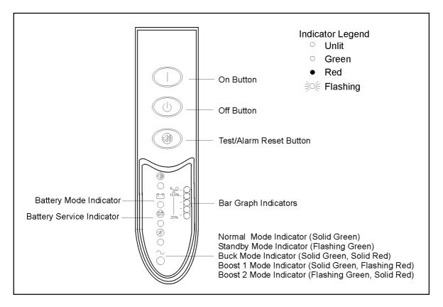
Figure 5. UPS Front Panel
